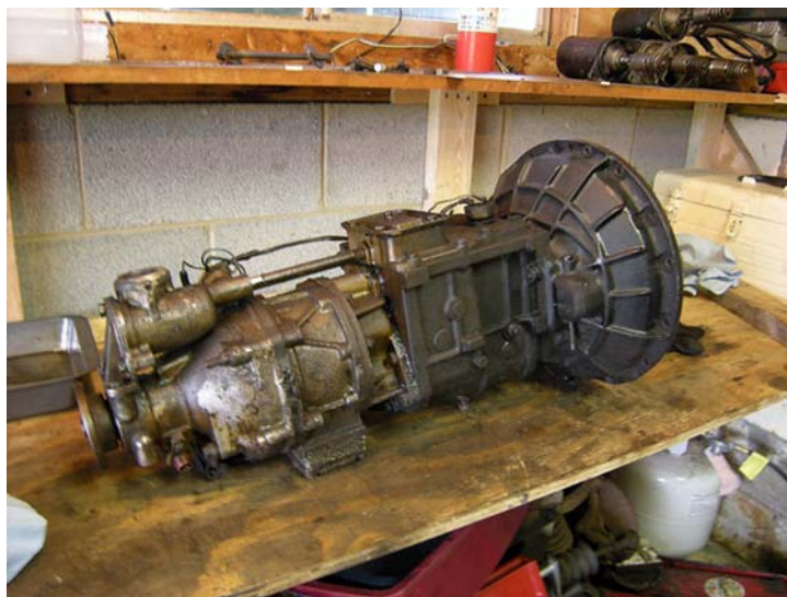
Below: The previously hidden overdrive transmission prior to being rebuilt
